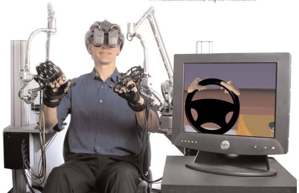
Figure 1: Haptic Workstation running the "Digital Seating Buck" application.
